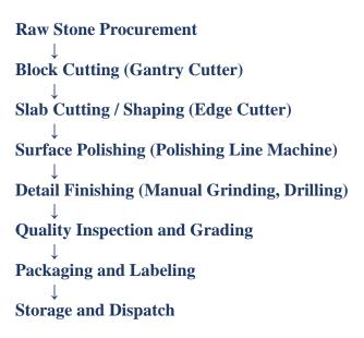
Each stage is handled with precision machinery and skilled labor. Wet cutting and polishing methods reduce dust and enhance the stone finish. Quality checks ensure each slab meets dimensional and aesthetic standards before packaging. Raw stone procurement from quarries
